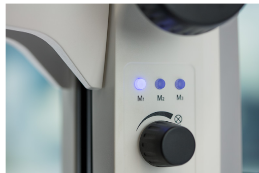
The memory section of stand M LED allows storing and quick recall of up to three customer specific illumination conditions. Press an "M" key long to store, press it short to recall your individual light scenario.
